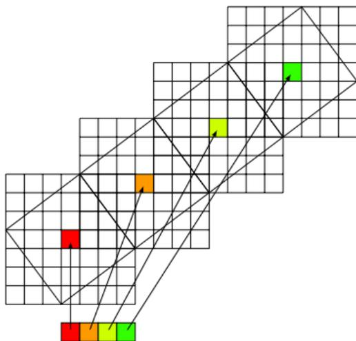
Connex pixels of the image are not connected (in the common sense) anymore after a  $(p, q)$  rotation, but are aligned on a  $(p, q)$ -directed line.
